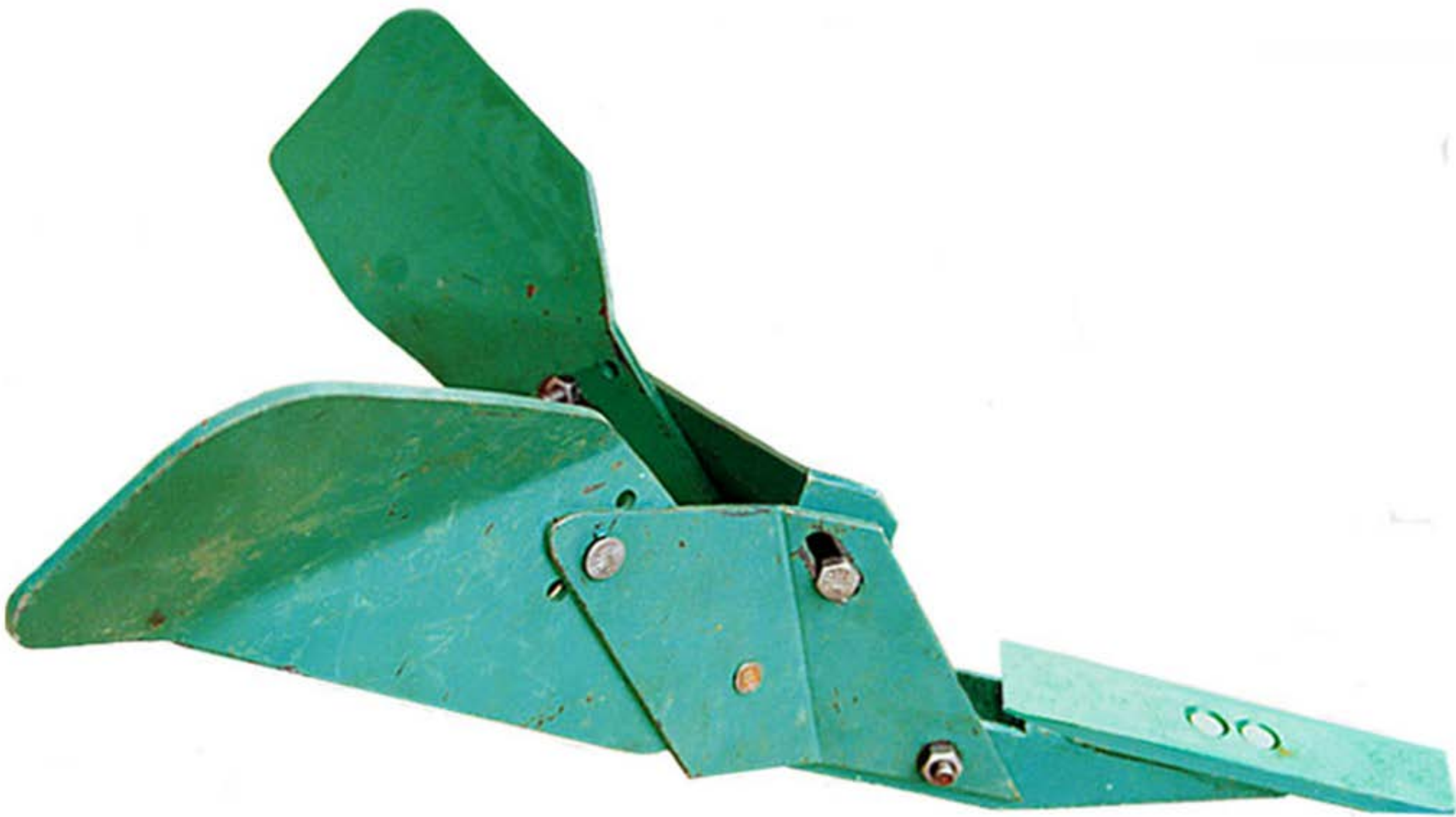
A deep winged factory design for a Magby gripper
