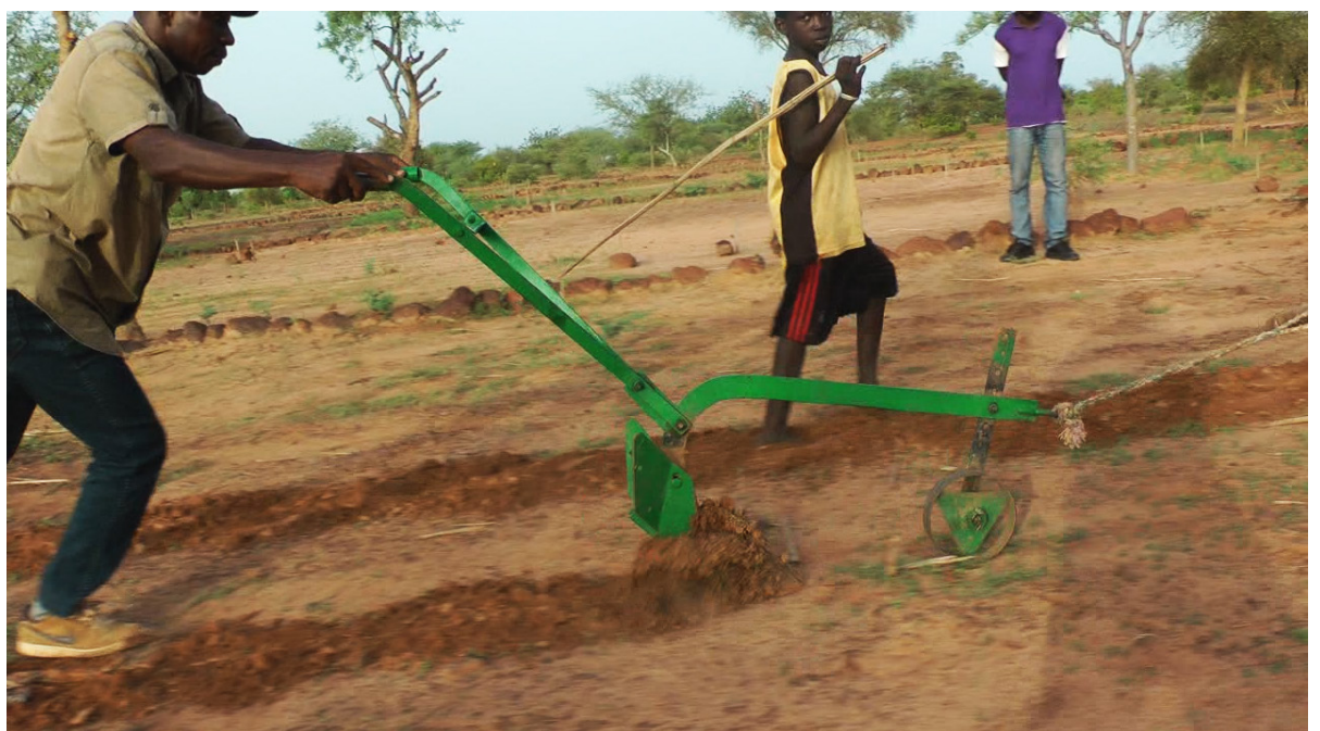
Land being prepared with a Magoye Ripper at a WAHARA field trial in Ziga, Burkina Faso (Image Courtesy: MetaMeta)
