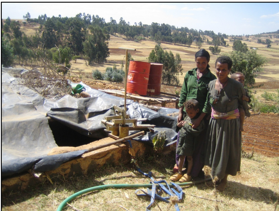
Figure 5. Treadle pump used for lifting water from rainwater harvesting tank to barrels
