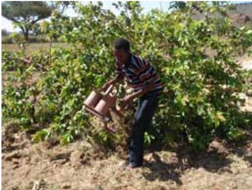
Figure 2. Using treadle pump to access the new shallow groundwater. Source: Tigray Bureau of Agriculture and Rural Development (Photo credit: Tigray Bureau of Agriculture and Rural Development, 2011).
