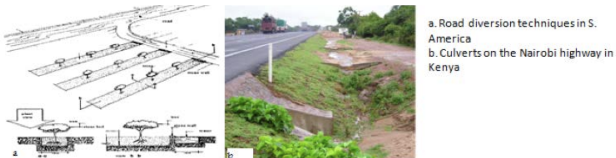
Figure 21: Road diversion systems and culverts for agricultural use.
